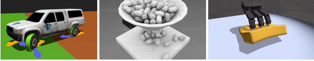
Fig. 35. The Matchstick model allows for control of frictional behavior in situations such as tire ground contact, a hopper, and soft robotic gripping, where each example shown here also uses different simulators with different contact solvers (Vortex, PROX, and Flex).
