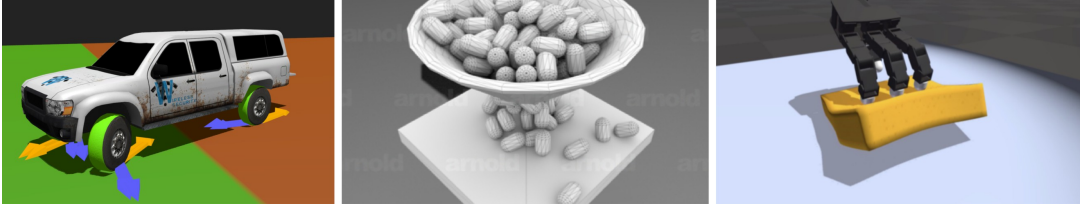
Fig. 32. The Matchstick model allows for control of frictional behavior in situations such as tire ground contact, a hopper, and soft robotic gripping, where each example shown here also uses different simulators with different contact solvers (Vortex, PROX, and Flex).
